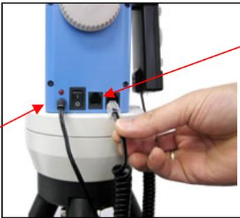
**Step 5. Plug in hand controller and AC adaptor.**
