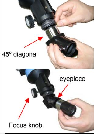
**Insert 45° diagonal:** Insert the diagonal into the eyepiece side of the telescope. Tighten the thumbscrews to a firm feel only.
