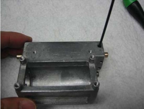
11. Remove the RA worm end cap. Push the end of the worm.
