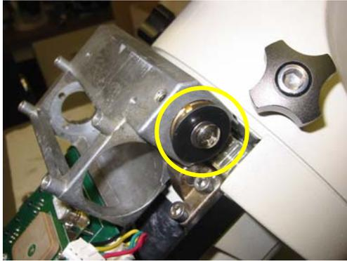
20. Turn the flat surfaces of the motor and worm gear shaft to face each other, so they can be easily accessed with the hex wrench after the wheels and belt are installed (see next step). You may power the mount on to rotate the motor shaft.
