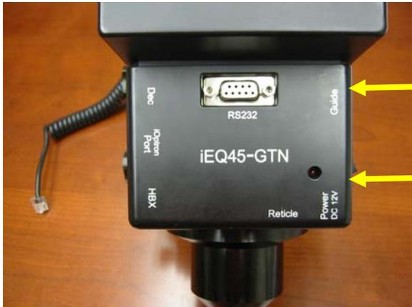
2. Remove black R.A. gear box cover by loosening the two screws.
