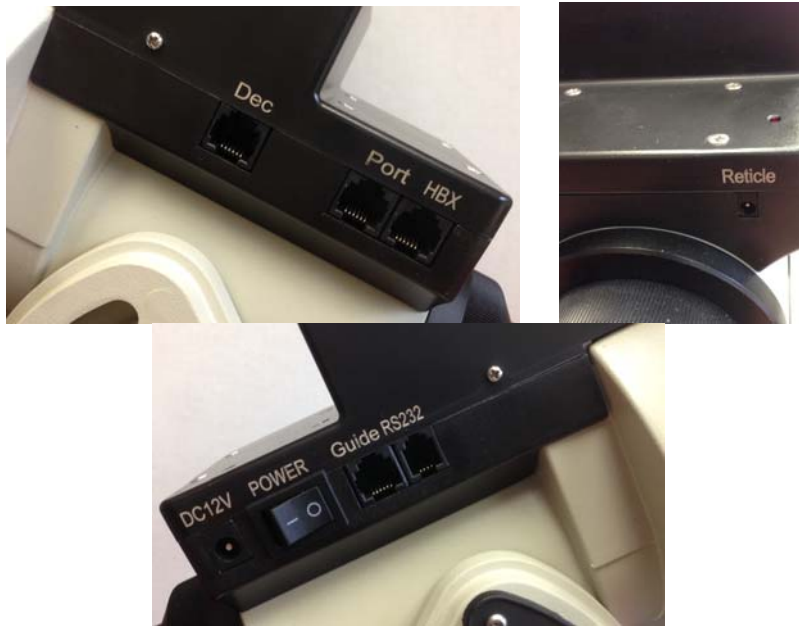
Figure 2. Ports on main control unit
