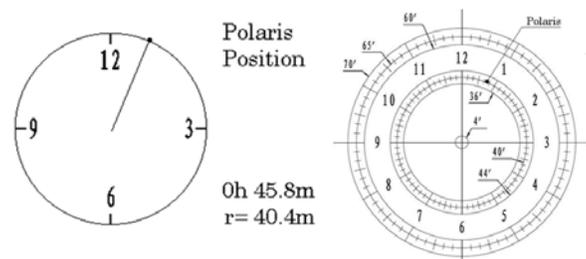
(3) Use the Azimuth and Latitude Adj. Knobs (not hand controller) to adjust the mount in both directions and put the Polaris in the location on the Polar Scope Dial (same as indicated on the HC LCD), as shown in the right side of the above figures.
