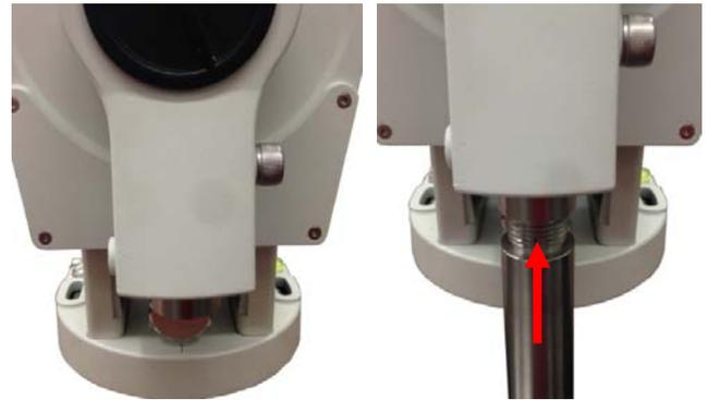
5. **Installing the Counterweight(s):** Before installing the Counterweight(s), make sure that both R.A. and DEC Gear Switches are fully engaged to avoid sudden mount movements, which could injure you or damage the mount gear system.
