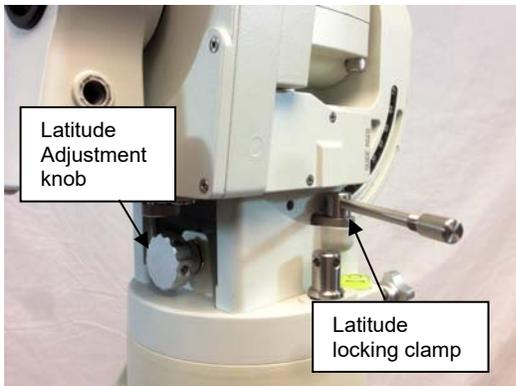
Turn the Latitude Adjustment Knob until the arrow points to your current latitude on the Latitude Scale. Tighten the Latitude Locking Clamps when done.
