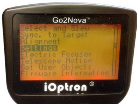
Before GPS pickup the signal (GPS OK), check for **Daylight Saving Time** using arrow key to toggle between **"Y"** and **"N"**. Enter the time zone offset to the UTC; for examples:
