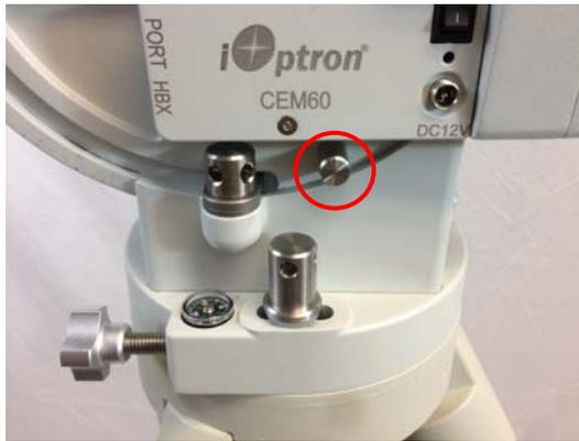
3. **Setting the Latitude:** Slightly loosen the Latitude Locking Clamps, use the SS lever if needed.
