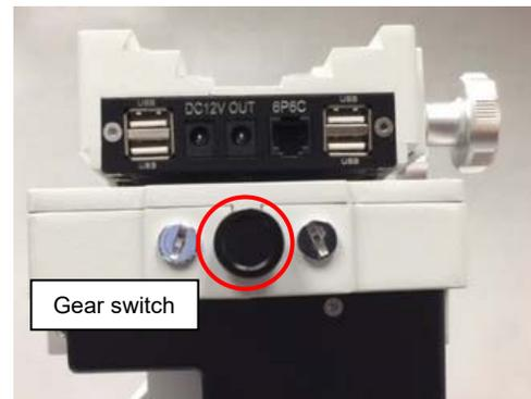
**CAUTION:** The telescope may swing freely when the R.A. or DEC Gear Switch is disengaged. Always hold on to the mount and/or telescope assembly before releasing the Gear Switches to prevent it from swinging, which can cause personal injury and/or equipment damage.
