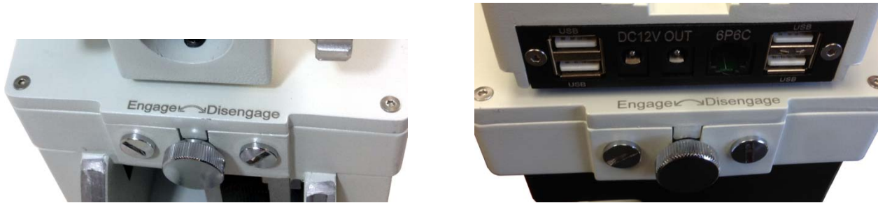
Figure 4. CEM60 R.A. (left) and DEC (right) gear switches
