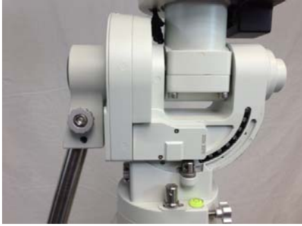
Figure 20. Tilt the counterweight shaft for low altitude
