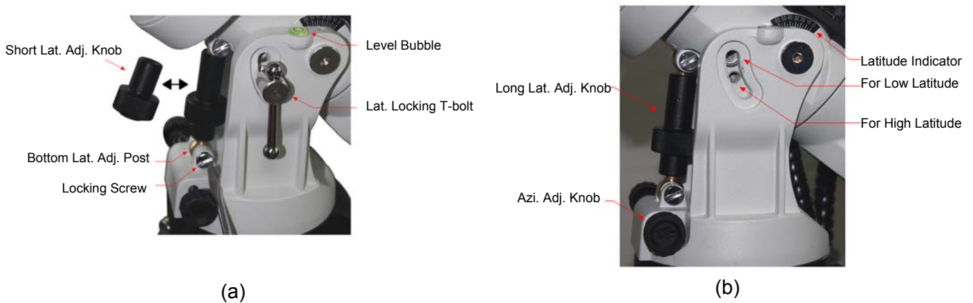
Figure 8. Switching latitude adjustment knob
