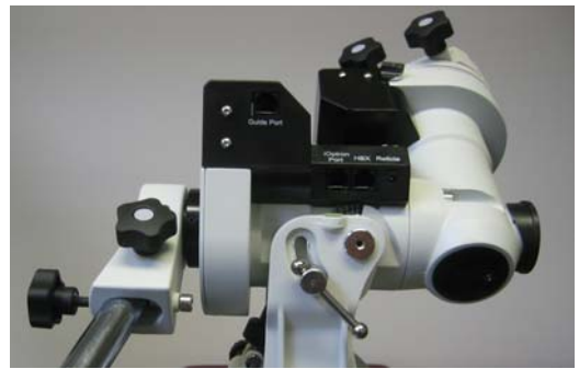
Figure 16. Rotate mount head 90° to clear the space for GPS receiver
