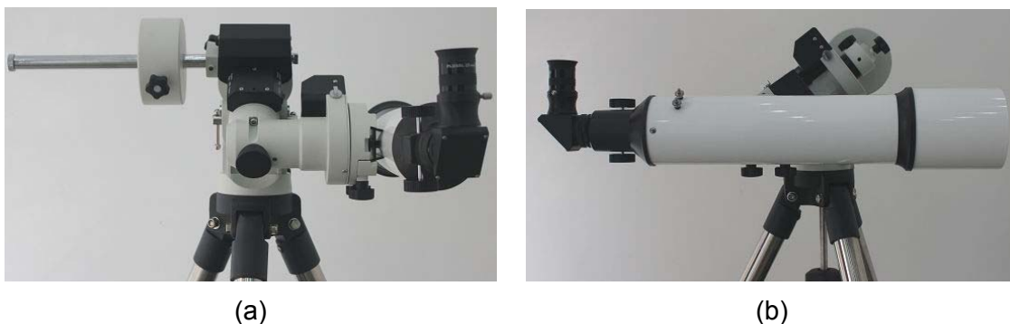
Figure 15. Balance along R.A. axis (a) and DEC axis (b)
