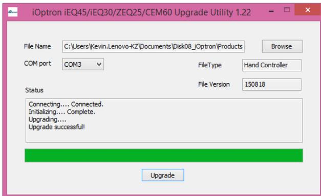
(8) After the firmware upgraded successfully, power cycle the mount. If no other firmware upgrade is needed, exit the Upgrade Utility program by click on . **Ignore any error message displayed on the hand controller if you need to upgrade R.A. and DEC control board firmware.** It will disappear after all firmware are upgraded.
