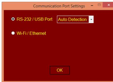
2. Select connection via RS232/USB Port, and choose Auto Detection. The iOptron Commander will automatic scan the system COM port and make the connection when click on OK button. If you know the assigned COM port, such as the native serial port will be COM1, you also can use the pull-down menu to select the COM port.
