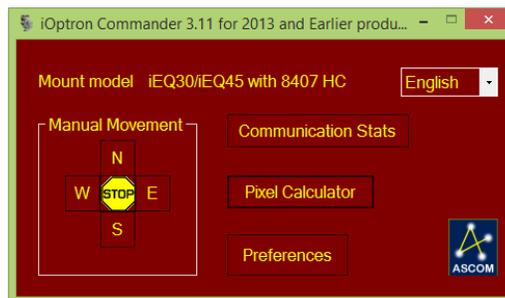
You may move the mouse to N,S,E,W and press the mouse to slew the mount.
